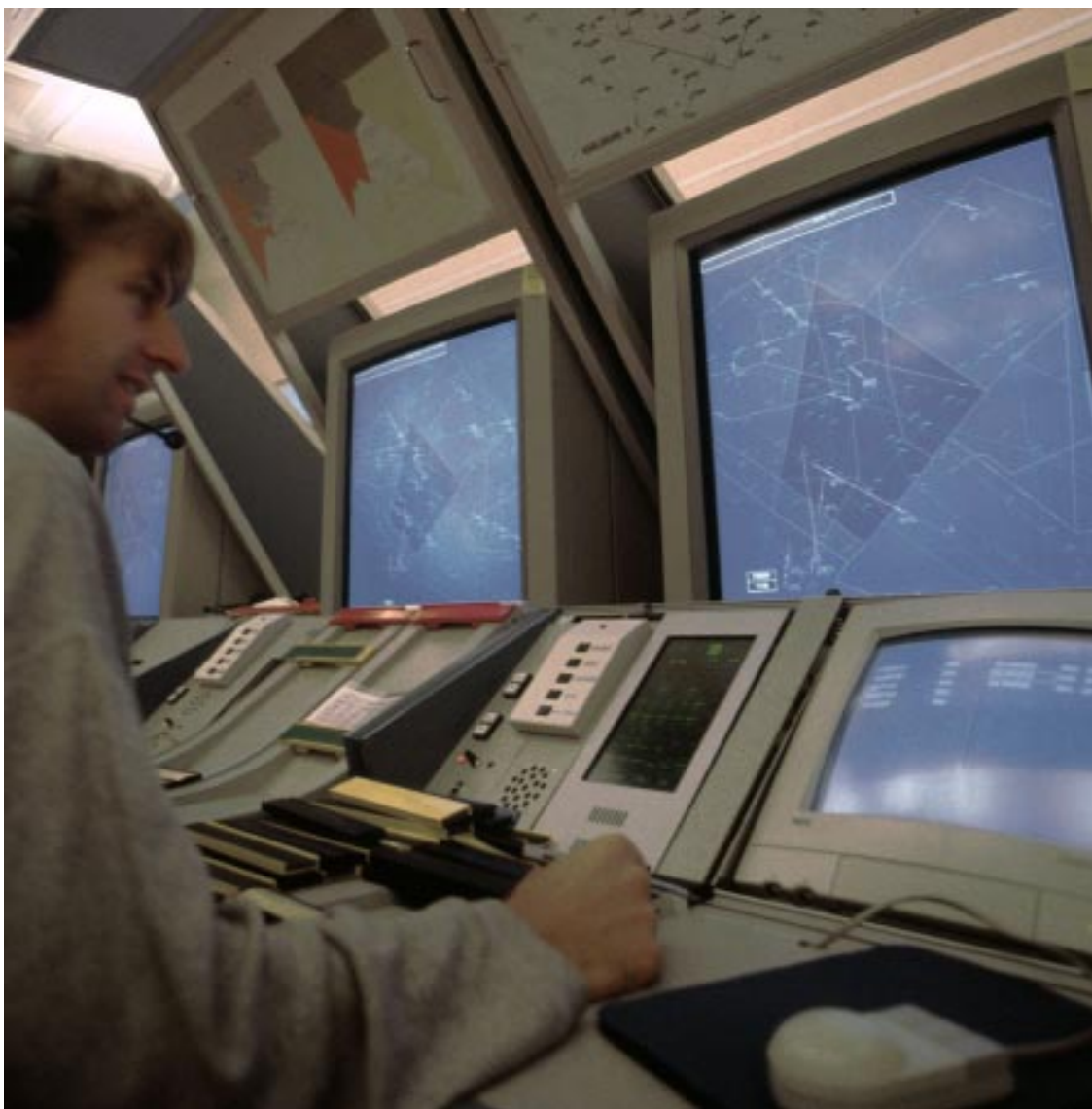
Figure 3: Controller Working Position (CWP)
